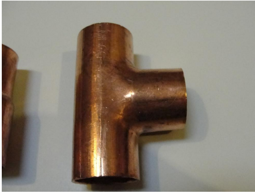
Tee to install onto piping
